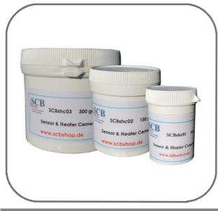
This cement is air curing and is ideal for mounting (potting) sensors and heaters. It's also usefull to protect the sensor and heater in your installation. It's easy to remove. Temp range from 1.5K to 1500°C. It has really good electrical insulating properties and is odourless.
