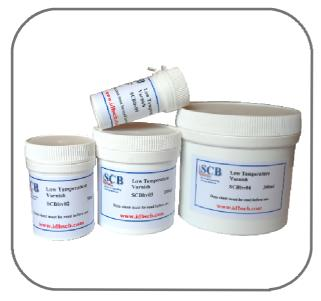
Former known as GE or IMI 7031 varnish. It's an air drying varnish (12-15 min) with excellent bonding properties and good electrical and chemical resistance. It's also for securing and thermally anchoring wires at cryogenic temperatures.
